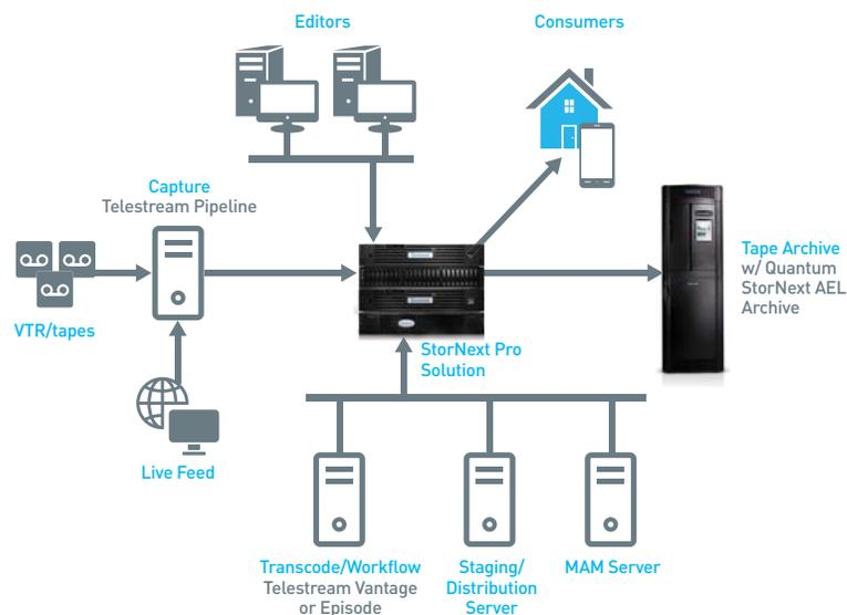
The combination of Telestream workflow and transcode products and the StorNext high-performance shared file system creates a powerful platform for enhancing workflow efficiency and performance. The example diagram above depicts a common broadcast workflow environment.
